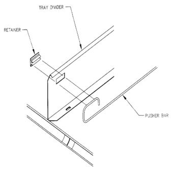
Figure 5.2 Pusher Bar Installation
